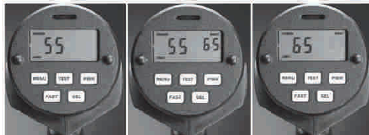
Figura 3.5.2 Modos Strongest Signal , Faster-Toggle y Faster-Hold .
